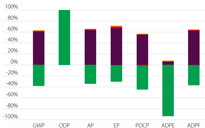
Figure 5 LCA results for structural hollow sections
